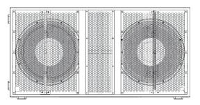
**BASSO** R218-A includes all the practical staples of live sound ground stacked, with handles and wheels positioned to facilitate load and setup, durable finish for metal and wooden parts, recessed front protection grill, vertical and horizontal wooden skates and a convenient front SpeakON NL-4 extra input.
