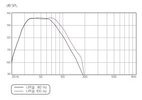
This graph shows the frequency response for a 1-watt swept sine signal in a semi-anechoic environement (2π), measured at 3 m and scaled down at 1 m.
