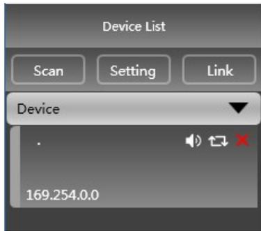
When using TCP control, there is a situation that only one point is displayed after scanning, but you can not connect to the device. In this case change the IP address of the device to the same network segment as the computer.
