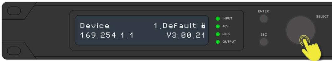
① Press **ENTER** or **SELECT** 5 seconds to unlock device, it will show menu list, turn the **SELECT** knob clockwise or counterclockwise to select functions: INPUT VOLUME, OUTPUT VOLUME, PRESETS, INPUT SOURCE, IP SET, RENAME, SECURITY. Press **ENTER** or **ESC** button to set function.
