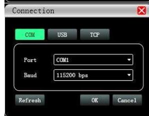
If you connect the device by using serial cable, click **Setting** in Device List, choose **COM** in Connection windows. Please check port and baud rate carefully for 232 before connecting.
