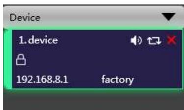
Successfully scanned and connected. Then click the device to load all parameters from the processor.
