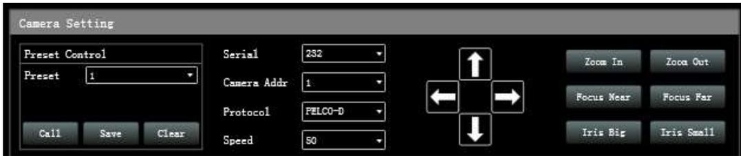
Generally, the camera position should be debugged before the tracking starts, and finally the parameter of this part are saved on the camera.
