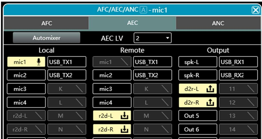
Matrix processor supports to control a certain degrees of echo from local room to remote room, which usually happened in remote video conference via network software Skype, Zoom, or via remote conference system controller(terminal). This function is mainly used for voice process.
