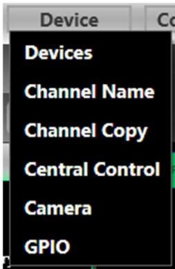
**Devices:** view or modify the software version information, device name and device IP address of the upper and lower computer of the device.
