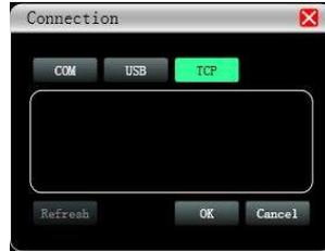
If you connect the device by using network cable, click **Setting** in Device List, choose **TCP** in Connection window.
