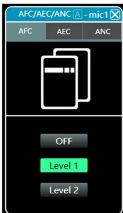
Matrix processor provides AFC (acoustic feedback control) function for microphone. With two level to select, user can control howl round easily when setting each microphone;
