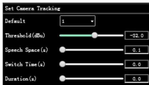
**Default mic:** when all mics have no input, turn the camera to the default MIC setting or send the associated command defined by the default MIC.
