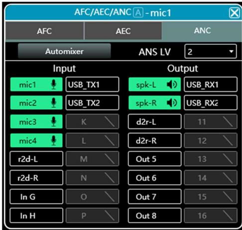
Matrix processor supports to control a certain degrees of noise, which comes from microphone, ground noise of input source, or surroundings. This function is mainly used for voice process.
