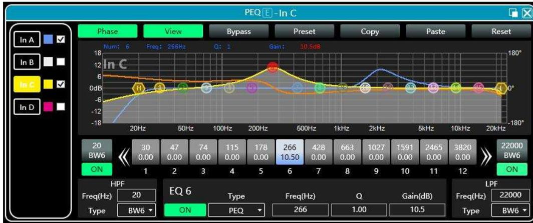
**Phase curve:** display the phase curve of the current channel.
