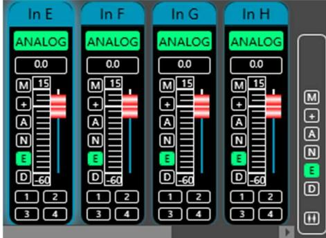
There are 3 kinds of input signal in device: ANALOG, Mic and testing signal. It will show a label for user.
