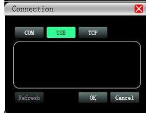
If you connect the device by using USB A-B, click **Setting** in Device List, choose **USB** in Connection window.
