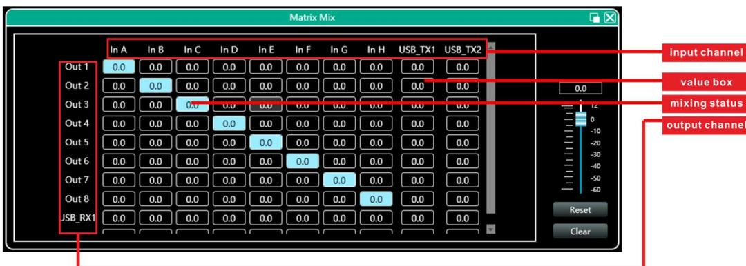
Input channel (on top side) corresponds to output channel. The box with a value is mixing key of channels. When the mixing key is cyan (double-click the value box to switch), the input channel and output channel signal realizes the mixing function.
