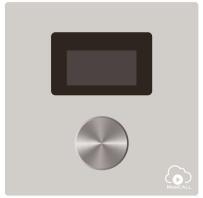
**MDM-CON1** is aPoE powered controller which communicates using UDP protocol. Fully configurable in the software, equipped with 1.31" OLED display. It offers various audio control capabilities such as volume adjustment, mixing, room combining and scene switching.
